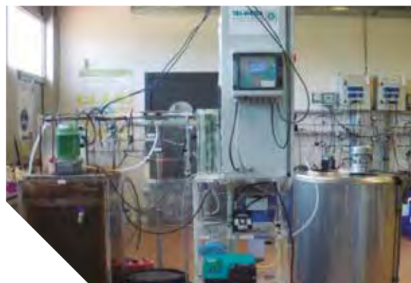
Fig. 1. Membrane bioreactor (Smart Air MBR) pilot plant (200L) for the treatment of greywater, being operated in the framework of the project demEAUmed.
