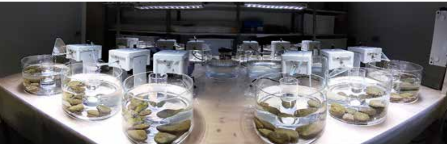
Figure 1 - Artificial mesocosms used for the exposure experiment of river biofilms to clarithromycin.
